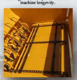
Bale Ejection Door: Patented side door opens sideways allowing for bale ejection if mold or unwanted material is discovered mid-process.
